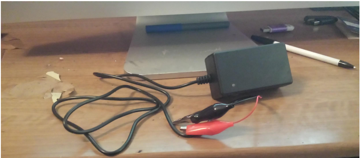
Fixed Output Power Supply (to negate argument that coil is drawing more power from battery to lift heavier load)
